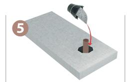
Fill in directly—no further formwork needed.
