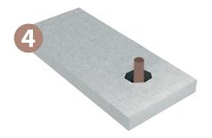
Run the service pipes through the opening.
