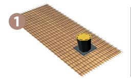
Cut away the rebars to position the box-out opening. Fit the RÉZABOITE CFO into place over the formwork base.
